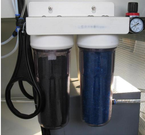
A photograph of a gas purification system. It consists of two vertical cylindrical towers, one black and one blue, mounted on a white base. A pressure gauge is visible on the right side of the unit. Various tubes and connectors are attached to the top and sides of the towers.                         |
