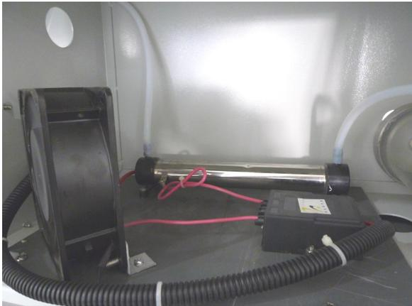
A photograph showing the internal components of an ozone generator. It features a dark, rectangular unit with a circular opening on the left, connected to a network of black and red hoses. A cylindrical metal component is visible in the background, and the entire setup is housed within a metallic chamber. |
